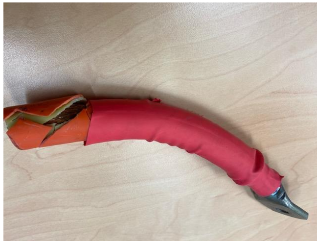
Figure 1: Degraded cable found in Hobart
