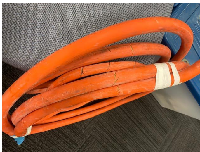
Figure 1: Degraded cable found in Hobart
