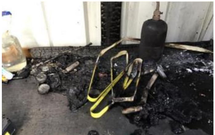
Figure 1: Remains of battery and charger on work bench following explosion
