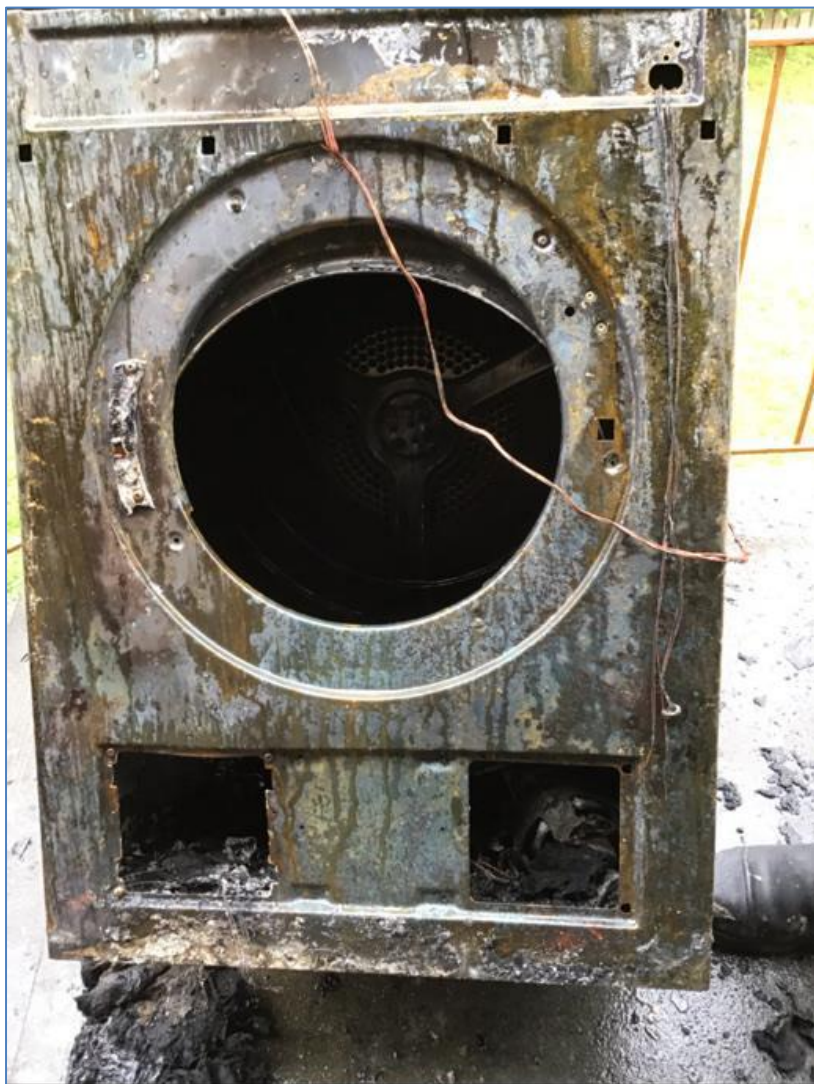
Image 3: Fire damaged tumble dryer
